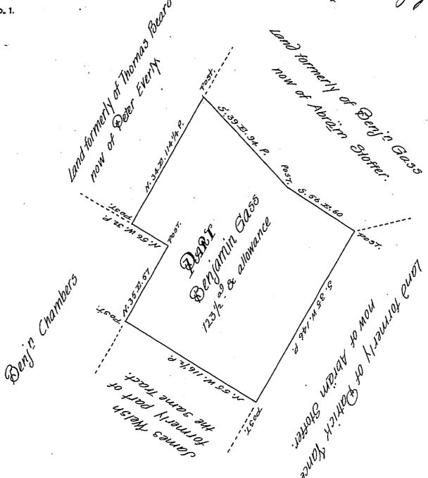
A Draft of a piece of Land situate in Guirford Township in the County of Franklin Containing one hundred & twenty three acres & an half & the allowance of Six P. Cent &c. being part of a Tract of 184 & allowance Resurvey in pursuance of an order of Survey granted to Benjamin Gass bearing—date the 5th September 1766 Nº 1125 Survey & laid off the above from the other part of Said Tract 32 December 1799.
